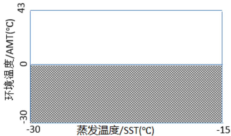
Pic.1 LT CDU Operation Envelope
